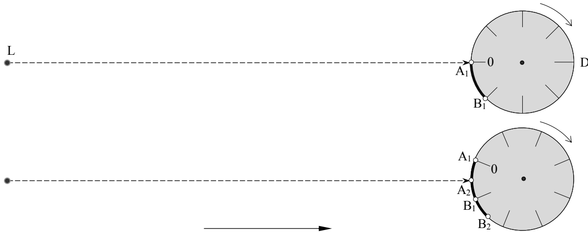
Fig. 4: Schematic of the experimental set-up: A_1 and A_2 denote the points where the rays generated by the first and the second light pulse hit the disk D at the instants t_1 and t_2 . The circular arc length A_1B_1 = d represents the trace on D 's photosensitive lateral surface the very first pulse causes. B_1B_2 = \omega \delta t_A depicts the trace's length increment produced by the second and any additional pulse according to the propagation hypothesis. The arrow at the bottom indicates the direction of motion of the earth around the sun.
